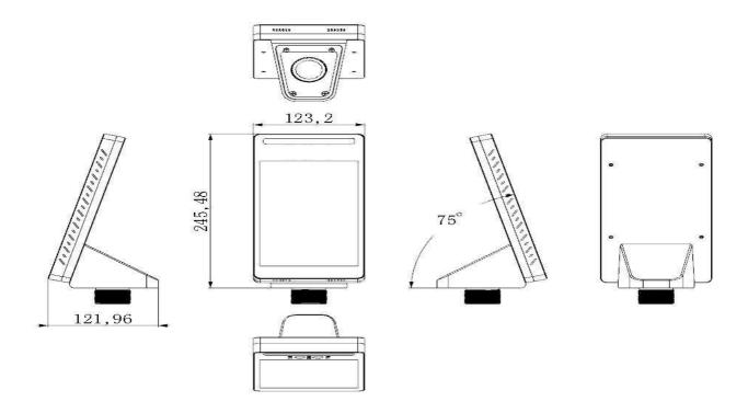
The opening has a circular diameter of 42 and is screwed to the screw base.
