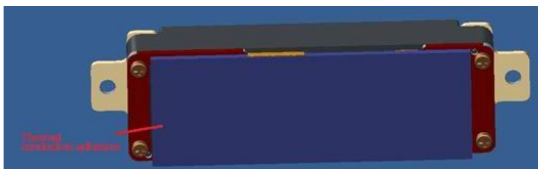
Installation location of thermally conductive silicone sheet
