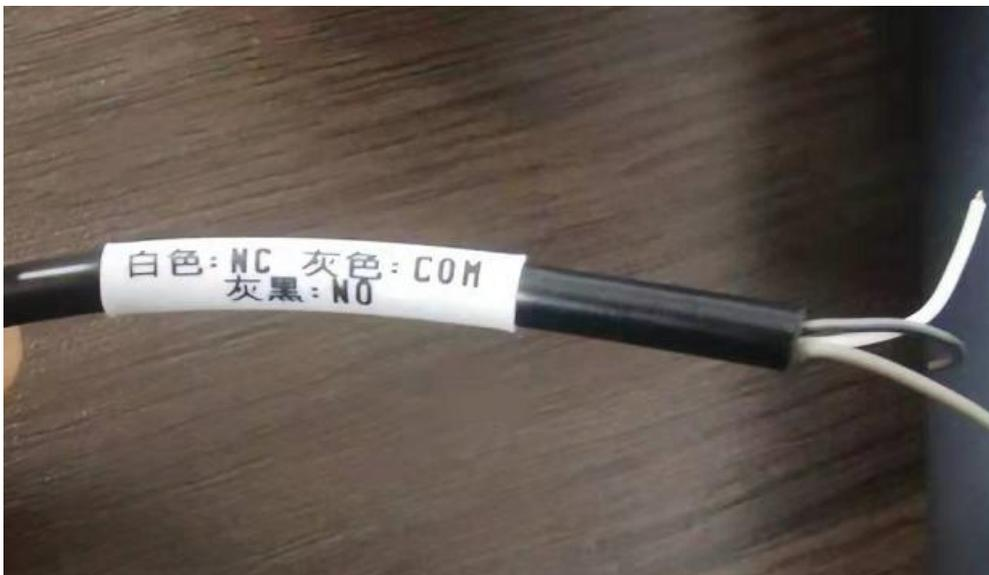
F6CS series products: 3P, COM and NO are respectively connected to the receiving and sending instructions of the gate. If the connection is found to be normally open or normally closed, the wiring is exchanged and tested.
