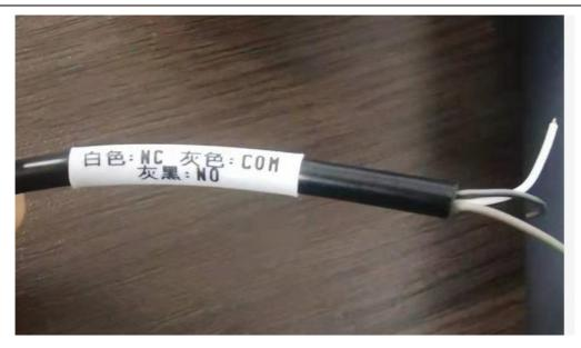
F6 series products: 3P, COM and NO are respectively connected to the receiving and sending instructions of the gate. If the connection is found to be normally open or normally closed, the wiring is exchanged and tested.
