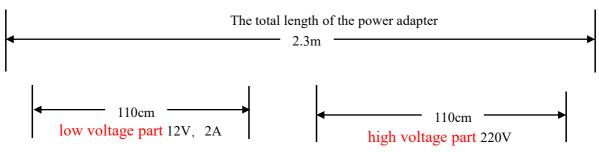
lead to insufficient power supply at the host terminal of the device, causing abnormal phenomena such as repeated restarts and crashes. If the power source is far away from the device, you can extend the power cord (high voltage part).
