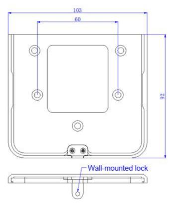
The wall mounted bracket supports standard 86 boxes of installation slots, and 86 boxes of machine screws are included in the package, which is convenient for construction and installation.
