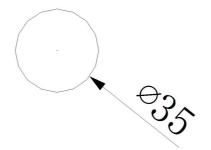
Requiring  $\varphi$ 35 hole, GB812 nut can be used to fix the column
