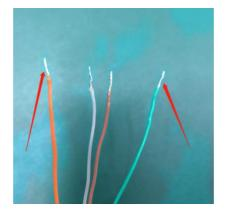
(2) Take out each screw, insert the wire head into the hole, fix the screw, test after locking to ensure if it is stable. Please check the picture below:
